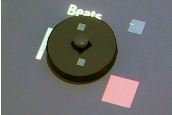
Figure 5: Our first approach to controlling the volume of a track in Audiopad. The puck is rotated to change the volume, just like a volume knob. The volume is displayed in a small bar graph to the left of the puck.
