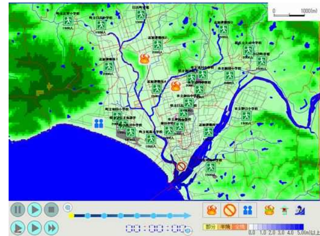
Figure 4: Screen image on the tabletop surface. Upper part is a workspace (a regional digital map). At the bottom of the table are simulation control buttons, a simulation clock and a menu of icons that can be added to the map.
