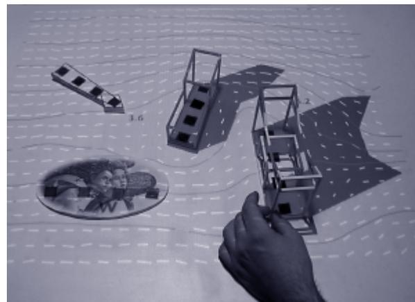
Figure 1: “Urp” urban planning simulation, with buildings, wind tool, and wind probe
