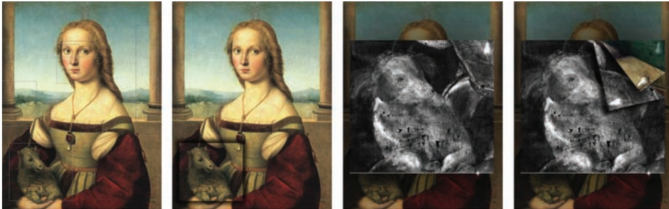
Figure 9. Our professional art diagnostic interface design. From left to right: faint outlines highlight areas of interest; selecting an area causes it to pop out of the background; the area expands to fill the screen and begins to fade between the uppermost layers; users can select which layers to fade between by turning over an image edge and selecting from the page corners (the page corner interaction is derived from the Fold n' Drop technique, see Dragicvic, 2004).
