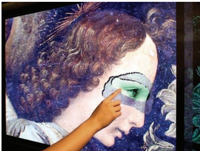
Figure 7. Wetpaint. Our first touch-screen interface for comparing multi-spectral scans of a painting uses the metaphor of scraping through layers to reveal the progression of the artist. The photograph shows two layers being scraped off by the user, as well as the page edges on the right of the screen used to navigate between scans.
