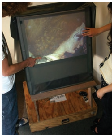
Figure 8. Our multi-touch screen prototype. This easel design was intended to offer a natural multi-user, ambidextrous touch interface that would complement a museum exhibit.
